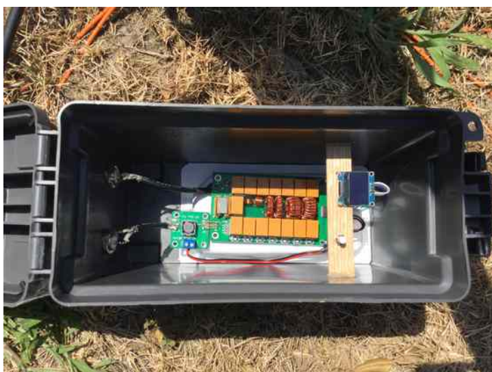
Illustration 1: AT-100 and Bias Tee temporarily hot glued to a plastic cutting board. Temporary wooden support is for a power reset button and OLED display.
